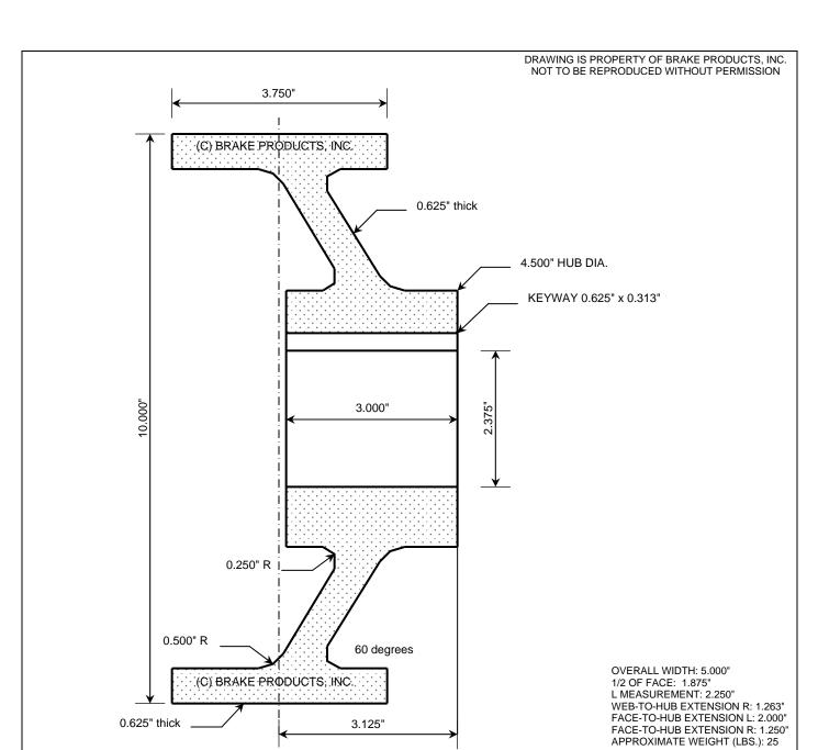
TOLERANCES: WHEEL DIAMETER: +0.005"/-0.000" BORE DIAMETER: +0.000"/-0.001"
